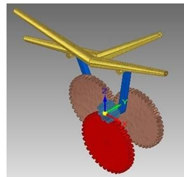
Figure 3: Wing mechanism
