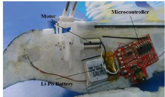
Figure 5: Complete assembly of MAV
