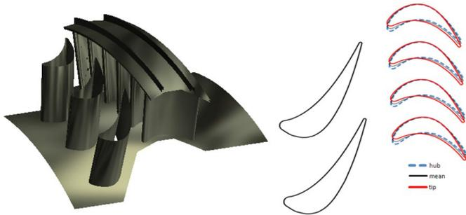
Figure 1: Geometry of the analysed turbine stage.
